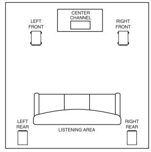
FIGURE 2 Alternate Loudspeaker Placement
